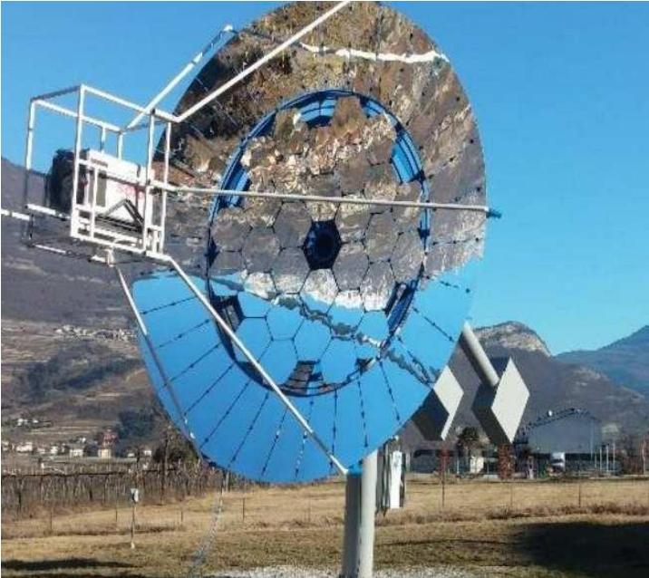
*Spherical and non-imaging optics to provide concentration ratios > 1000 suns.*
