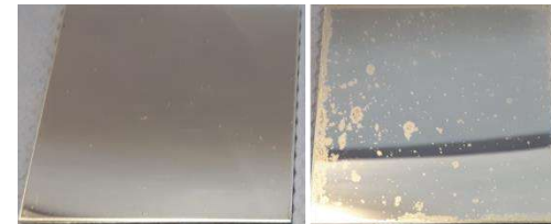
Mirrors with and without PECVD coating after 2 weeks in damp heat test
