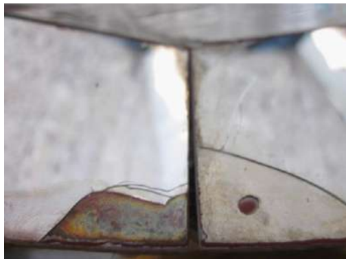
Edge corrosion and glass breakage of water cooled secondary reflector after 14 months in operation at PSA
